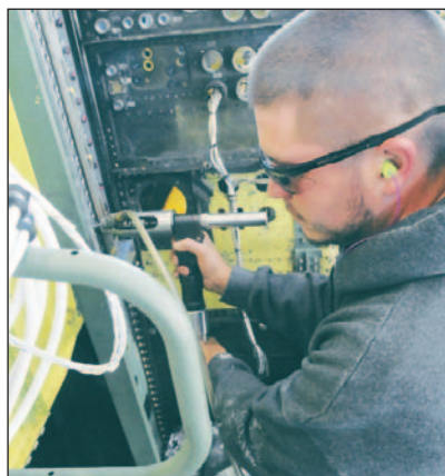
Dustin Dykes, sheet metal mechanic, drills the main beam support for a new center wing box. Any C-130 aircraft the Air Force does not plan on retiring before 2046 will undergo CWR.
