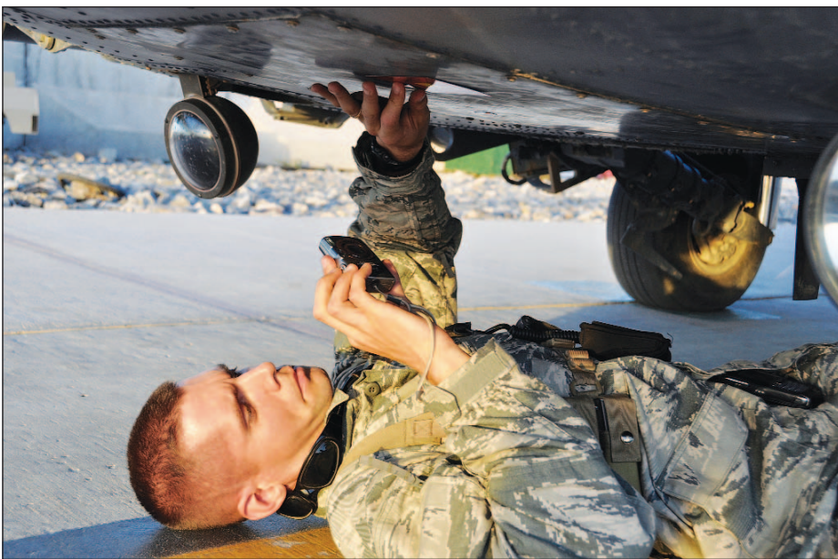
U.S. Air Force photo by TECH. SGT. RENNI THORNTON Capt. Mark Friesen, Joint Combat Assessment Team member at Kandahar Airfield, Afghanistan, takes a photo of a bullet entry point on an HH-60G Pave Hawk. The helicopter had received enemy small-arms fire during a rescue mission.
