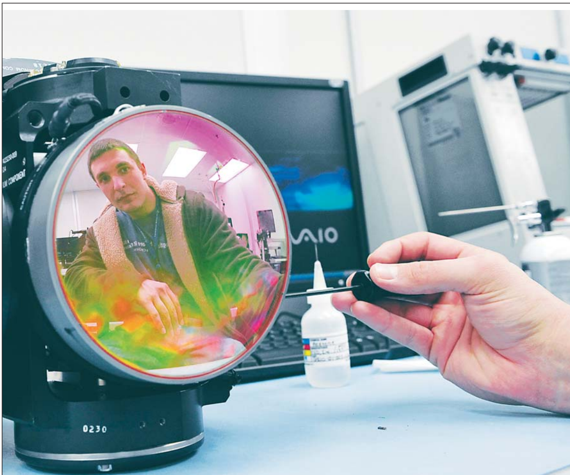
U.S. Air Force photo by TOMMIE HORTON Tyler Barfield, an electronics technician in the 402nd Electronics Maintenance Group, performs optic alignment and adjustment procedures on the rotating gimble assembly of a Sniper XR Advanced Targeting Pod.
