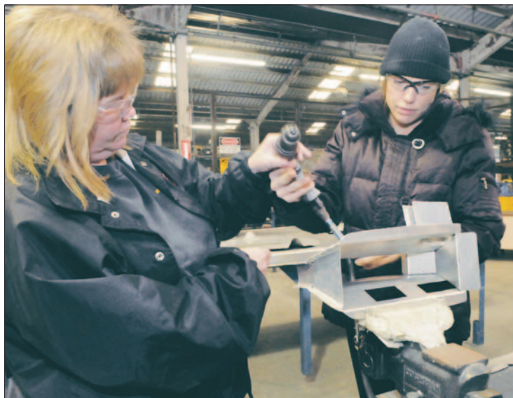
Kristen Barwick, left, and Cozette Peebles, fabricate a B-29 armament chute.
