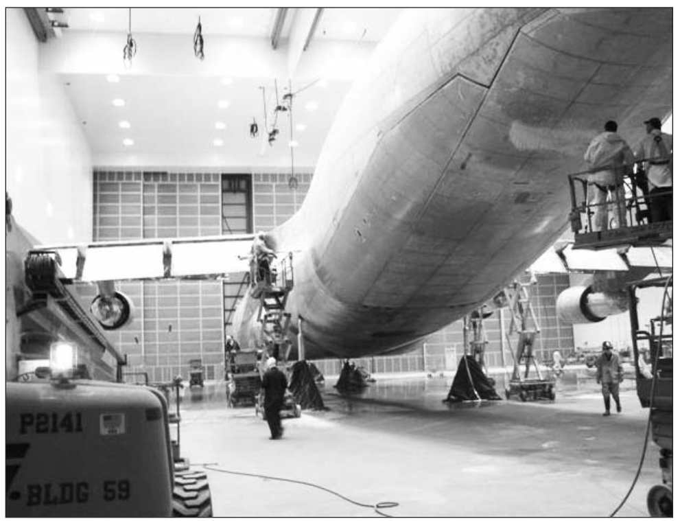
402nd Maintenance Wing workers apply the PreKote Surface Pretreatment to a C-5 Galaxy.
