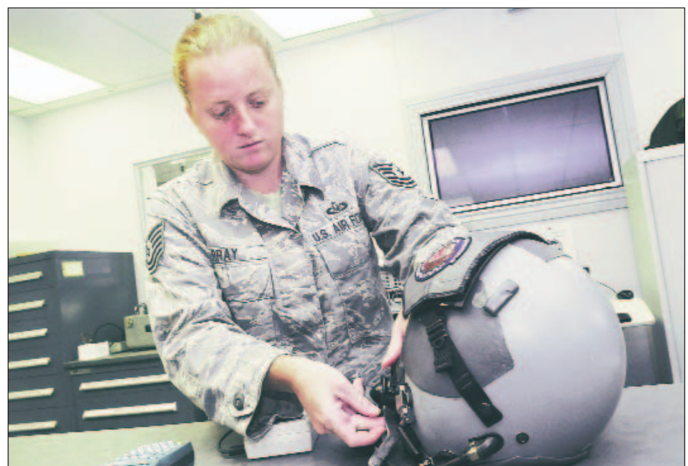
Tech. Sgt. Brandi Bray, aircrew flight equipment technician, checks the microphone and headset and does a calibration check on a helmet.
