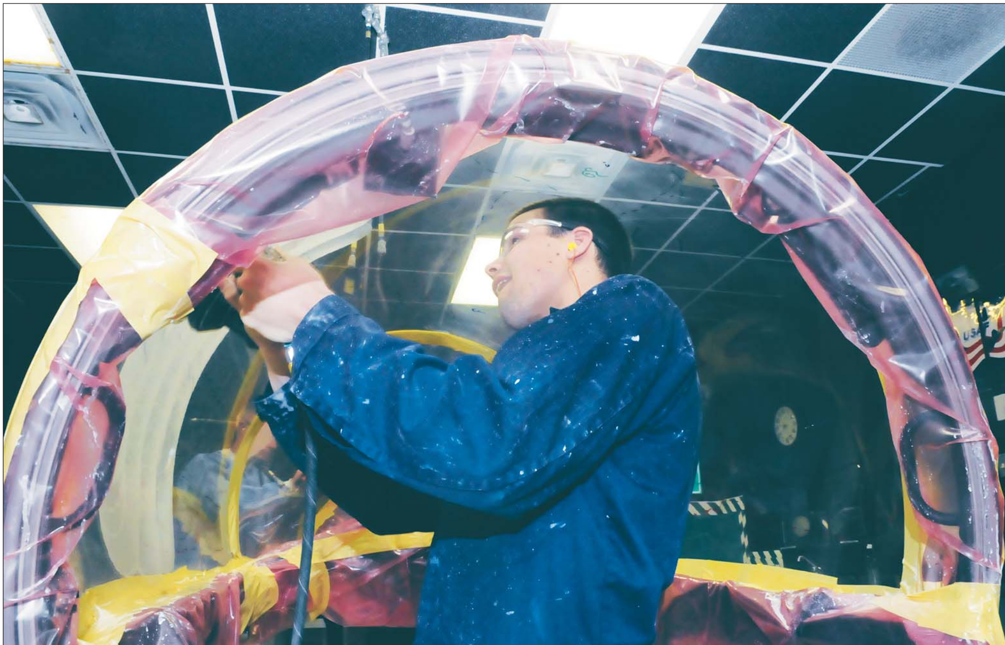
Staff Sgt. Roy Nunn, Oregon Air National Guard, polishes the inside of an F-15 canopy. Sergeant Nunn is here as part of a training program. Aircraft maintainers from around the world visit the shop for an 80-hour course to get certification in canopy polishing.
