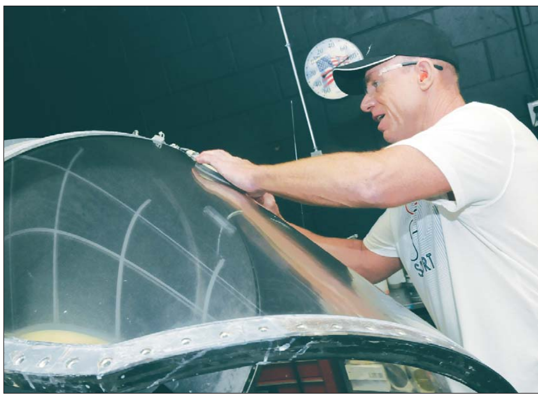
Above, Chris Jones, a mechanic in the 561st Aircraft Maintenance Squadron, reconditions a wind screen for an F-15 in the canopy shop.
