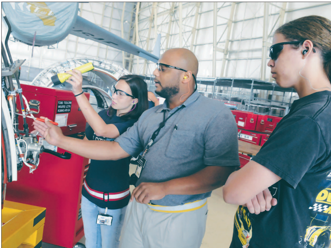
Jeffrey Williams, center, shows high school seniors Heather Kearns and Ryan Fenimore how an inspection is done on a C-17 engine thrust reverser. The inspection is done to check for cracks, leaks, and wear and tear.
