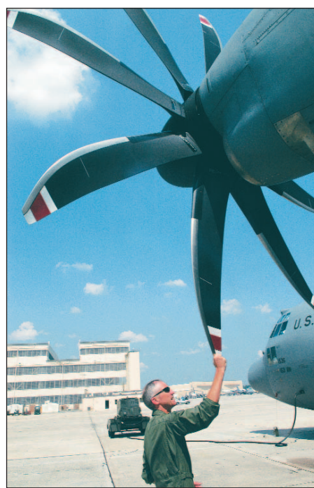
Col. Dennis Grunstad, 153rd Air Wing commander, talks about the improvement the eight propellers make in the capabilities of the C-130 H3.
