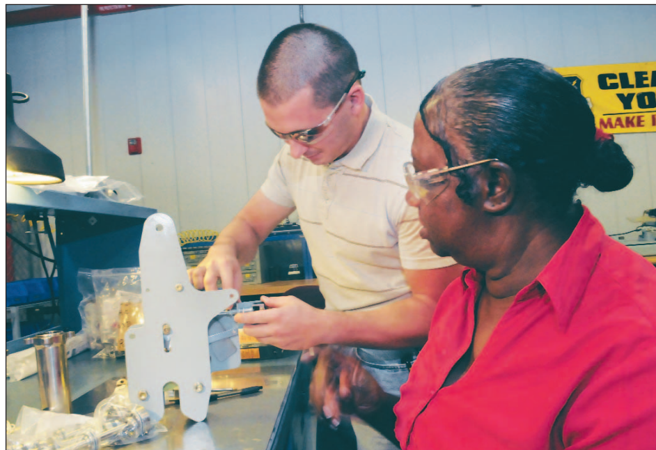
Mark Windham and Rosa Jordan, pneudraulics systems mechanics, work on a C-130 air cargo door uplock.
