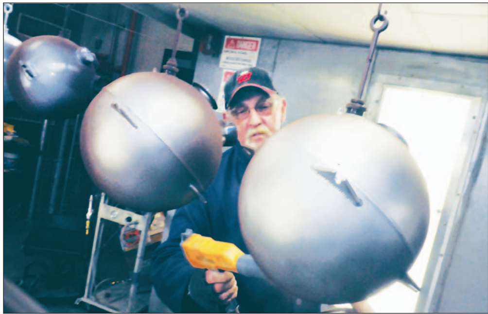
Gary Henderson applies a powder coating finish on fire bottles.
