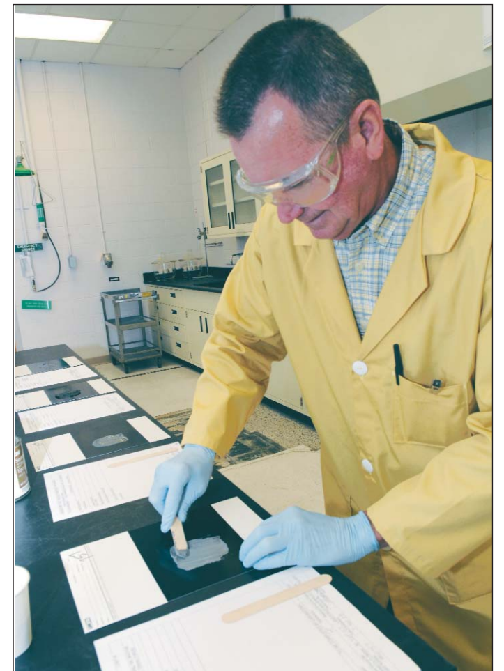
Mike Butts, chemist, performs cure testing to determine if a product is still usable. The cure time can vary from 30 minutes to 22 days. The shelf life testing saved $1.1 million in fiscal 2008
