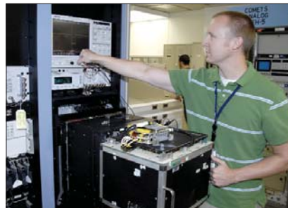
U.S. Air Force photo by CLAUDE LAZZARA Michael Hunt, lead test station operator, prepares to test the first production asset using VDATS, a decoder assembly from the Pave Penny pod.
