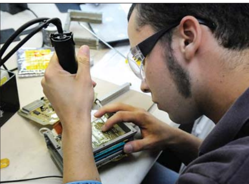
Below, Steven Pierson, electronics technician, repairs solder joints on an A-9 decoder card for the Pave Penny pod.
