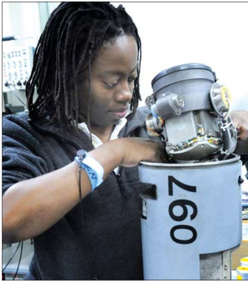
Natalie Clett, one of the original Votech employees, troubleshoots and replaces damaged parts on the Pave Penny pod, a targeting device used on the A-10 Thunderbolt II.
