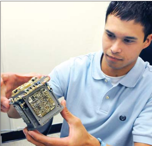
Above, Willard Fox shows the receiver system of the Pave Penny pod.
