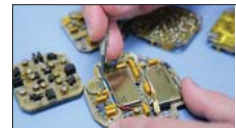
Circuit cards have to be repaired to ensure the Pave Penny pods can accurately illuminate targets.
