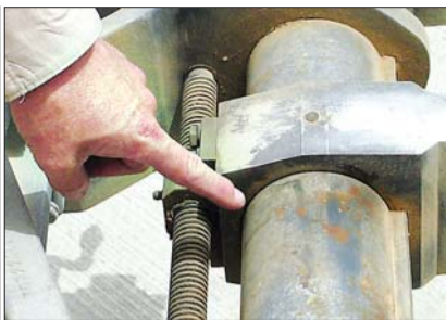
Surface corrosion excess dust and sand accumulation is pointed out on a C-130 aircraft tow bar.
