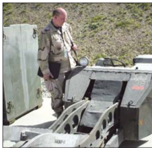
Rob Cooke, corrosion team member, evaluates a munitions bomb lift for corrosion and weathering.
