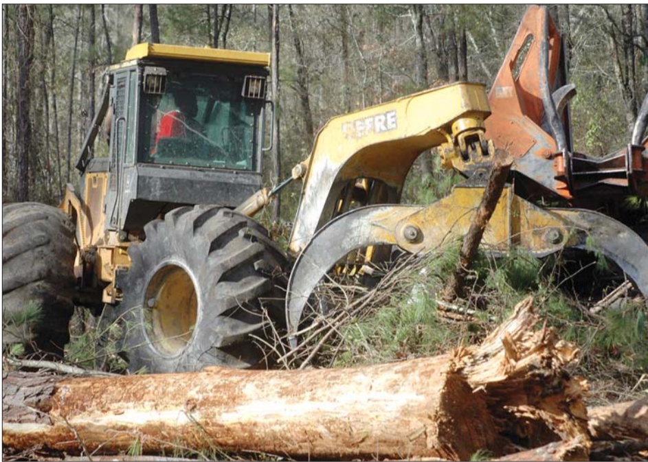
A skidder drags downed trees to be loaded and picks up debris.
