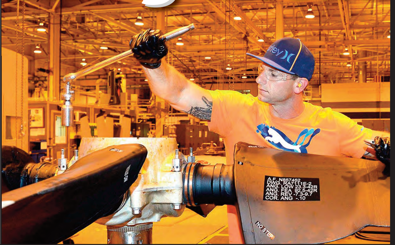
Steven Vann, 572nd Commodities Maintenance Squadron aircraft propeller mechanic, tightens barrel bolts on a C-130 propeller prior to testing. Propellers make their way through five gates, or work processes, at the Warner Robins Air Logistics Complex.
