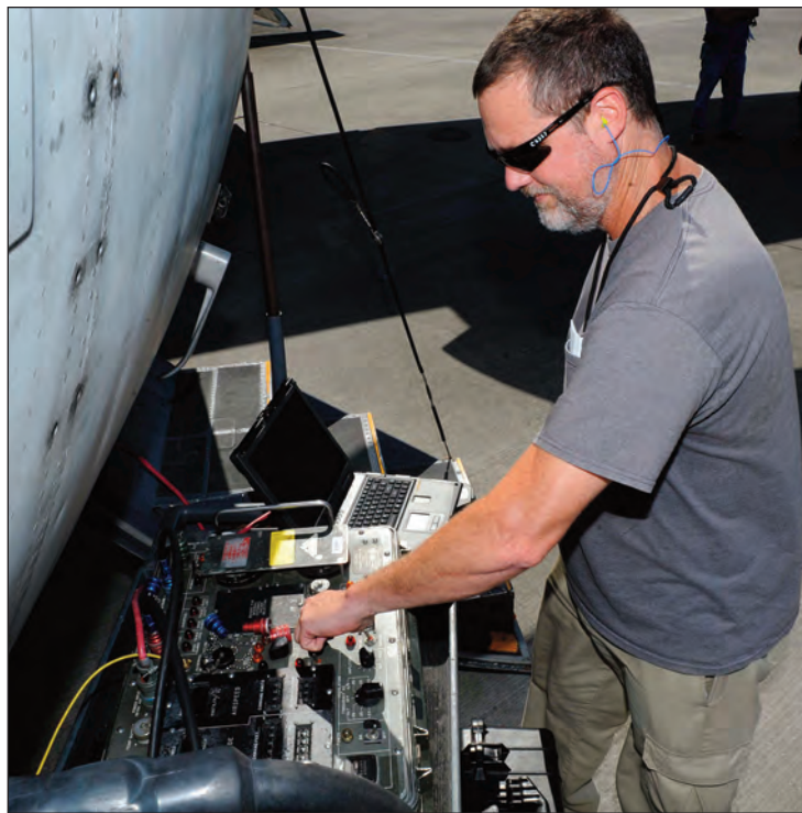
U.S. Air Force photo by TOMMIE HORTON Chris Cashell, 560th Aircraft Maintenance Squadron work lead electrician, performs indicator static checks on a Coast Guard C-130H.
