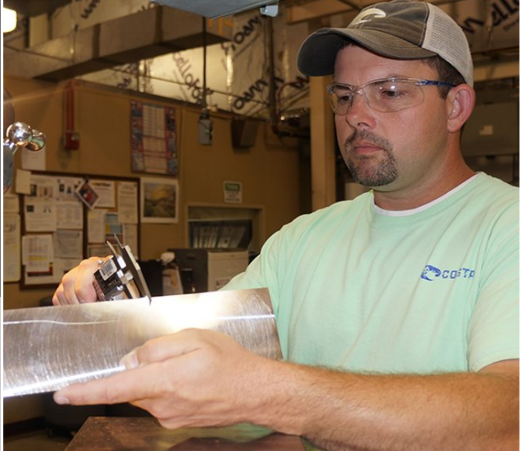
Daniel Yarbrough, 402nd EMXG machinist, uses a pair of calipers to make sure the aluminum he has milled meets blueprint requirements. (U.S. Air Force photos/ED ASPERA)
