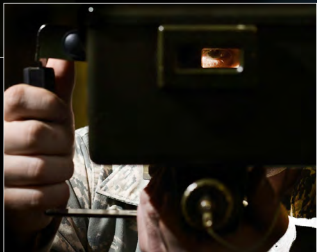
Above: Airman 1st Class Jordan Johnson, a 380th Expeditionary Aircraft Maintenance Squadron avionics specialist, verifies the integrity of an RQ-4 Global Hawk antenna, using an identify friend or foe transponder. The IFF antenna allows other aircraft to recognize the Global Hawk as a friendly aircraft.
