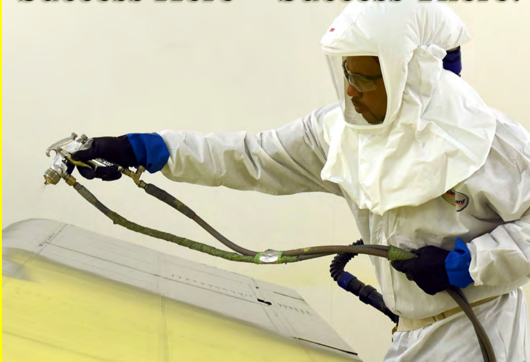
Rivers Foreman, 571 st Commodities Maintenance Group aircraft painter paints a C-130 and C-17 aileron inside an enclosed paint booth at the organization's paint/depaint facility. Three newly installed paint booths in Bldg. 180 have helped the organization drastically reduce production times, work hazards, health hazards and environmental impact simultaneously. (U.S. Air Force photo by Tommie Horton)
